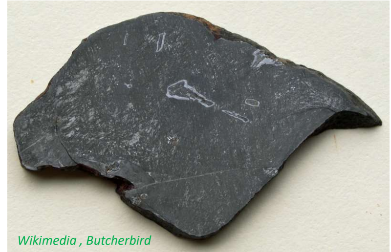
slice of the Gebel Kamil Meteorite with schreibersite rimmed by kamacite
