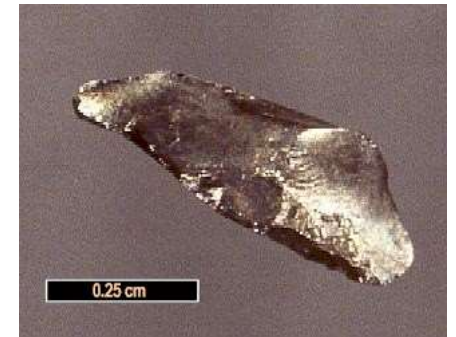
slice of the Gebel Kamil Meteorite with schreibersite rimmed by kamacite
